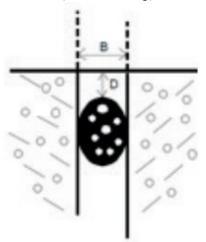
Materials used as backer rods should be weaker that the sealant itself and not obstruct the movement of the sealant, whilst compressing or expanding. Most suitable backer rods are:
